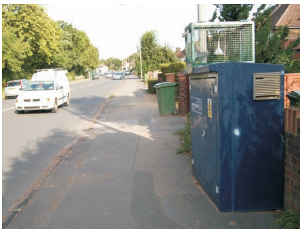
Temporary monitoring station installed as part of a programme to improve air quality in an AQMA
