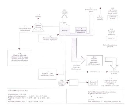
Figure 4.1: Solvent Management Plan Inputs and Outputs
