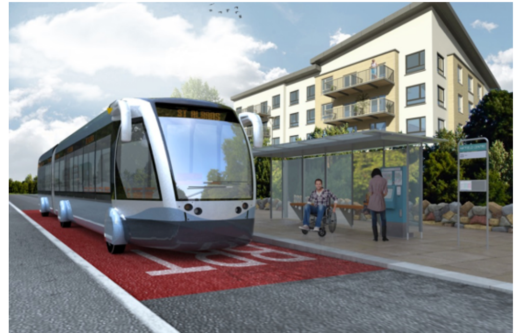
Fig. 13: Bus Rapid Transit concept - Vehicles benefit from being able to operate on segregated guided tracks as well as on roads, therefore offering greater route choice and flexibility than heavy or light rail options.
