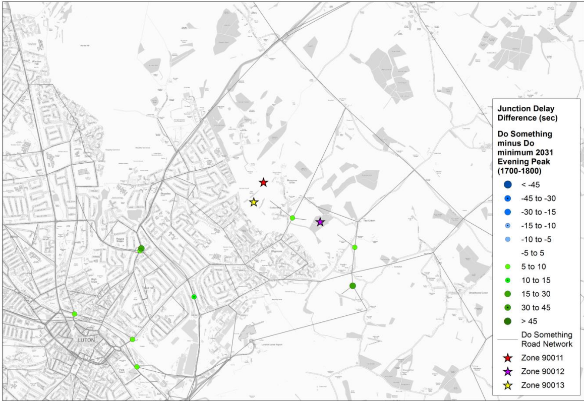
Figure 14 – Junction Delay Difference Plot (2031 Do Something minus Do Minimum) (Evening Peak Hour)
