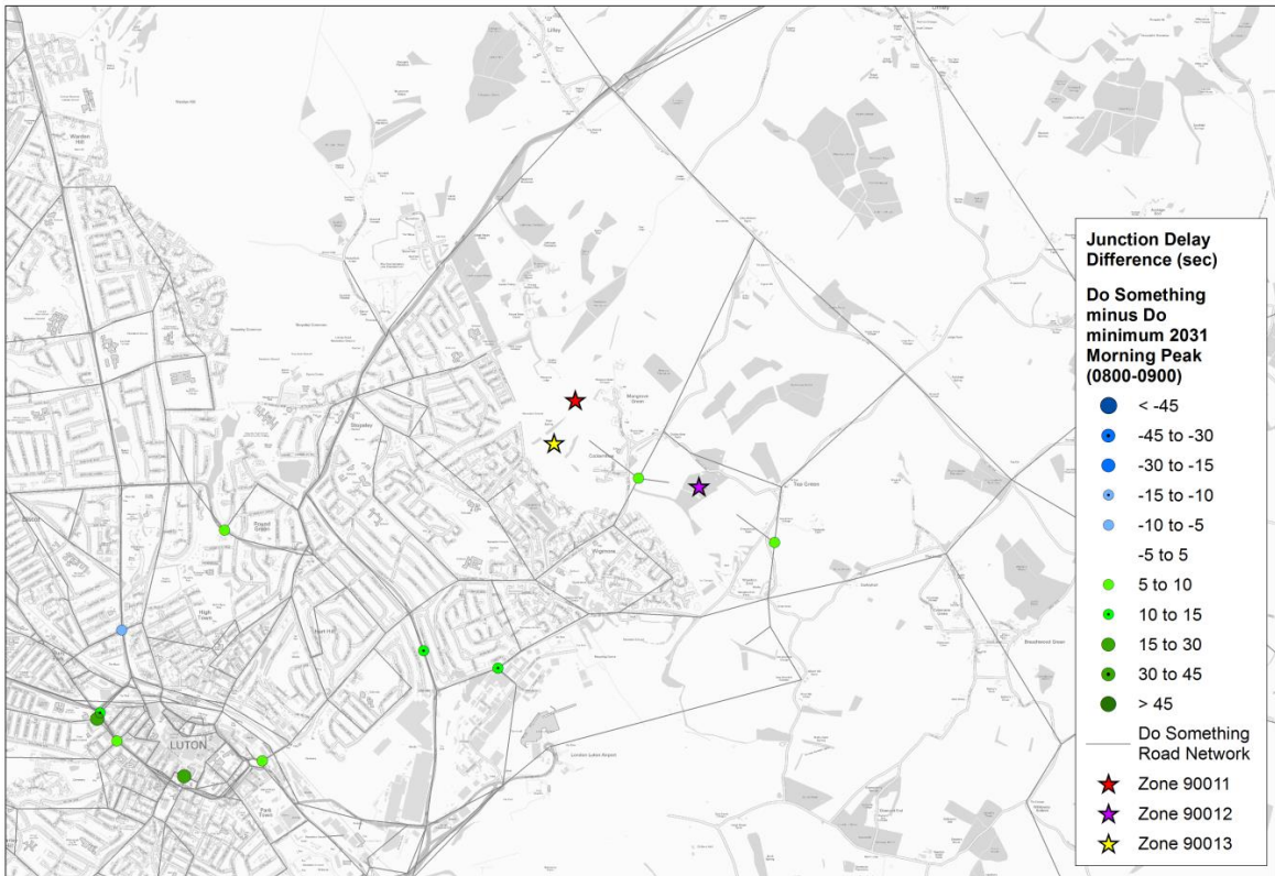
Figure 13 – Junction Delay Difference Plot (2031 Do Something minus Do Minimum) (Morning Peak Hour)
