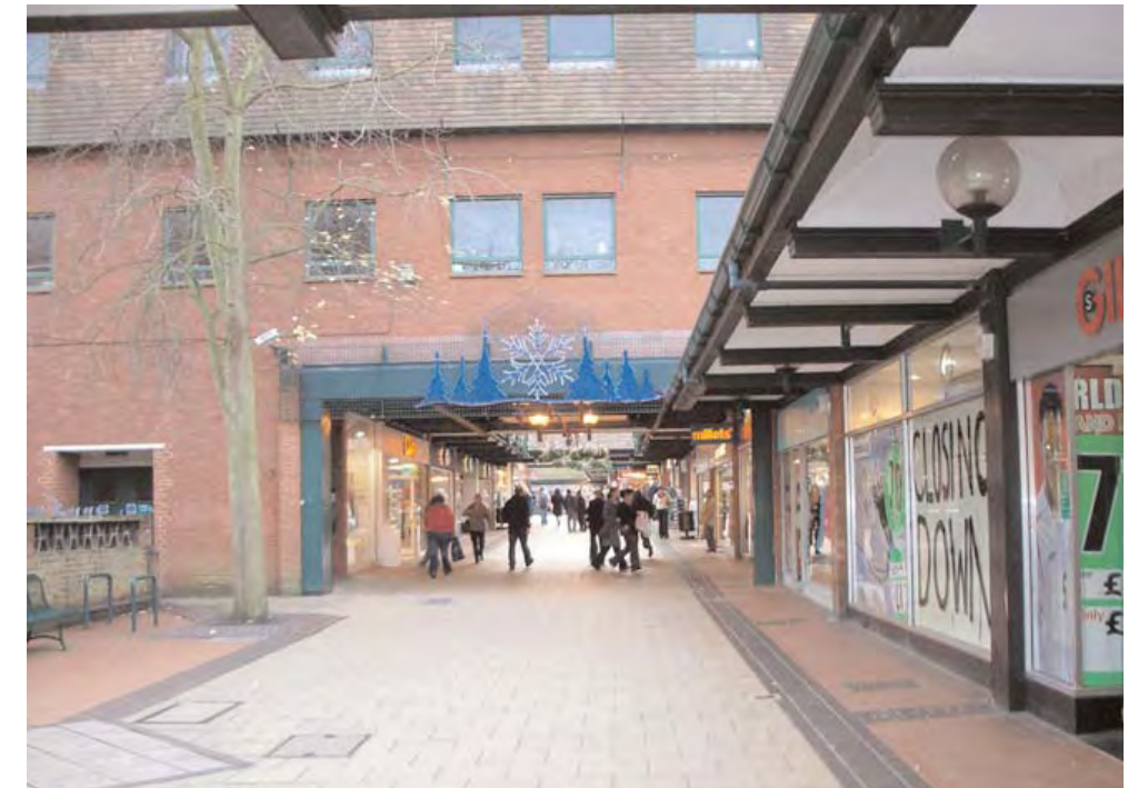
2. Garden Square shopping centre is dark due to the low canopies and dark brick.
