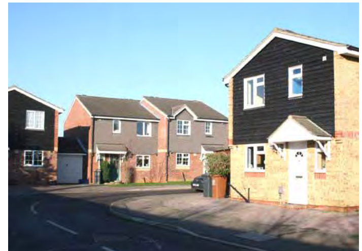
12. Housing at Talisman Street in the Post-war Suburban zone, showing light yellow brick and black timber cladding. Porches have tiled canopies.
