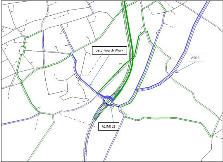
Figure 3.6 Detail of flow differences in the Pirton Road / A505 area in Hitchin
