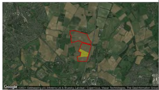
Observer Location Sun azimuth range is 270.2° - 290.3° (yellow)
