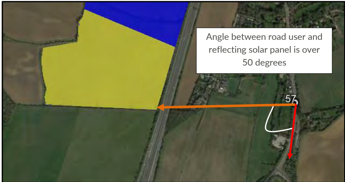
Figure 28 Aerial image showing the bearing from location 57 towards the reflecting solar panel area
